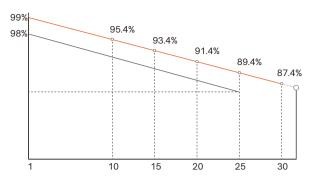
DAH Solar linear power output guarantee \_ - Standard linear power output guarantee
